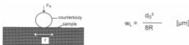
Fig. 4 Pattern of the oscillation wear test (Ref 1)
